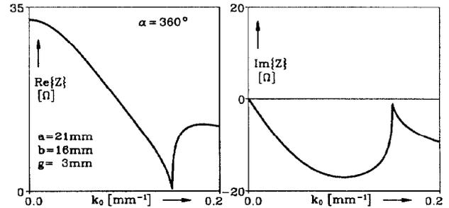
Figure 7: impedance for  $\alpha = 360^\circ$
