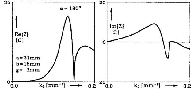
Figure 5: impedance for  $\alpha = 180^\circ$
