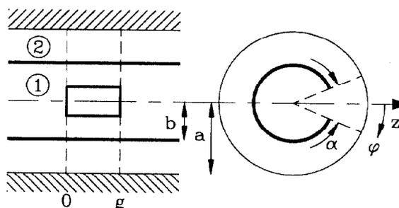
Figure 2: coaxial waveguide with a rectangular hole in the inner conductor
