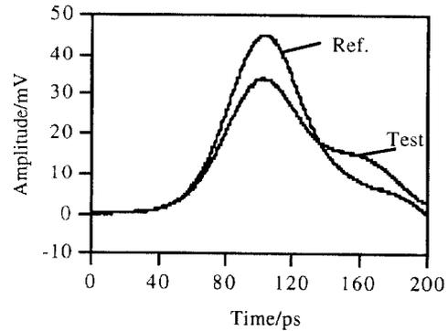
Figure 4. Gaussian Pulse Data for a D-Quadrupole Loss Parameter Measurement
