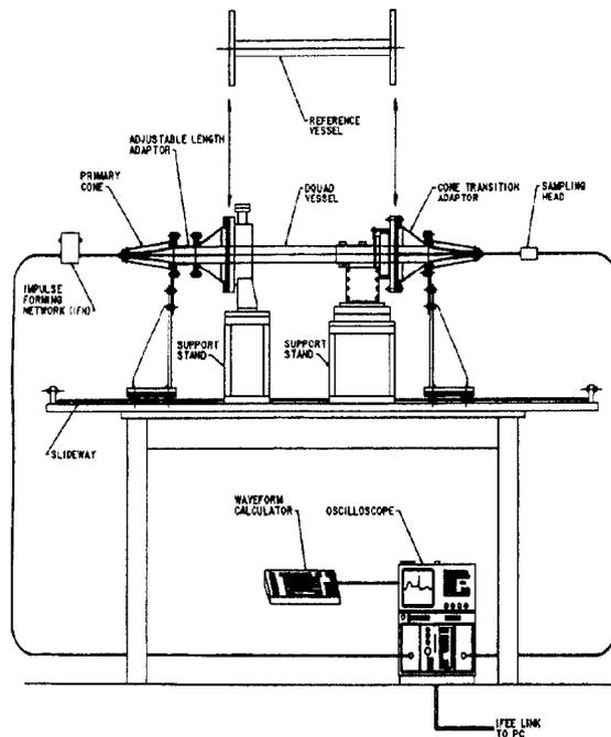
Figure 5. Layout of New Impedance Measurement Rig.
