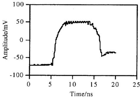
Figure 2. TDR Data from Reference Vessel
