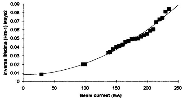
Figure 2. Instantaneous lifetime against beam current
