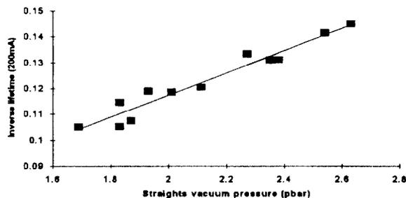
Figure 4. Development of lifetime and pressure during first period (5 days) of high current running.
