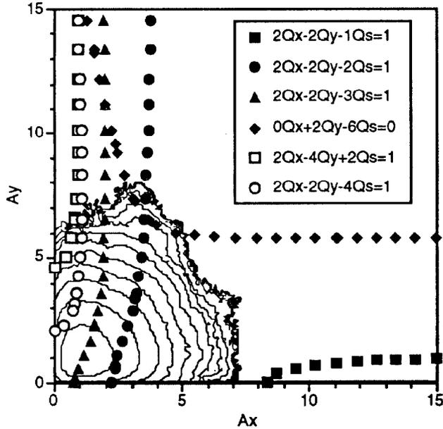
Fig 1. LEP beam-beam tail distribution and resonances. A linear, symmetric lattice is used. The tunes in the legend refer to 1/4 of the total tunes.
