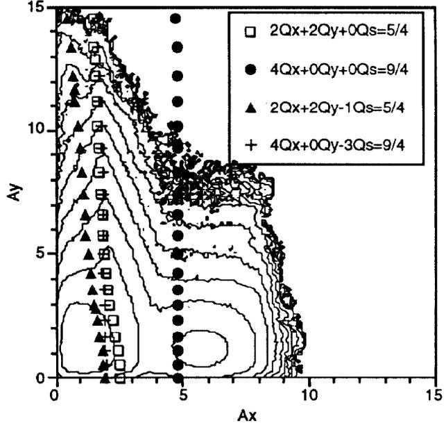
Figure 2. LEP beam-beam tail distribution with lattice including errors. The tunes in the legend refer to 1/4 of the total tunes.
