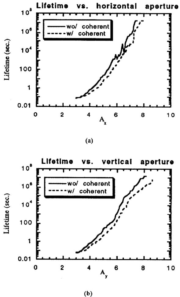
Figure 5. Lifetime as function of (a) horizontal and (b) vertical aperture, with and without strong beam coherent motion.
