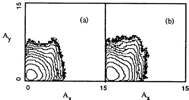
Figure 4. LEP beam-beam tail distributions. (a) without coherent motion; (b) with strong beam quadrupole mode coherent motion.
