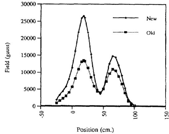
Fig. 1 - Field profiles for the old and new design
