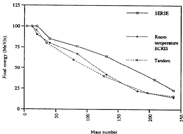
Fig.3 - Cyclotron energy for different injectors.
