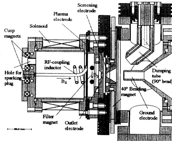
Fig. 8 Schematic drawing of the source and the extraction system.
