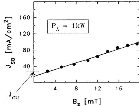
Fig. 4 Extracted current density as a function of solenoidal field strength. ( $p_s = 15Pa$ )
