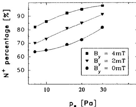
Fig. 3  $N^+$  percentage as a function of source pressure. ( $I_A = 10A$ ,  $U_A = 100V$ )
