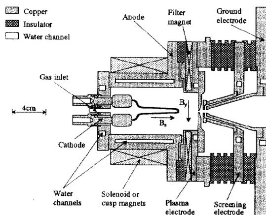
Fig. 1 Schematic drawing of the source and the extraction system.
