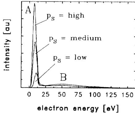
Fig. 5 Electron energy spectra for three different source pressures.
