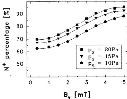
Fig. 2  $N^+$  percentage as a function of transverse magnetic field strength. ( $P_A = 1kW$ )
