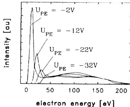
Fig. 6 Electron energy spectra for different plasma electrode potentials.
