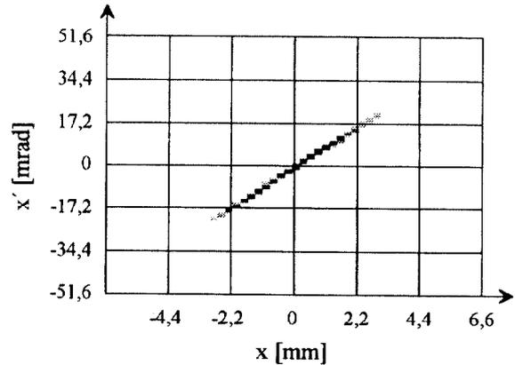
Fig. 7 2D-emittance diagram of the extracted beam. ( $U_{EX} = 17\text{kV}$ ,  $I_{EX} = 9\text{mA}$ ).
