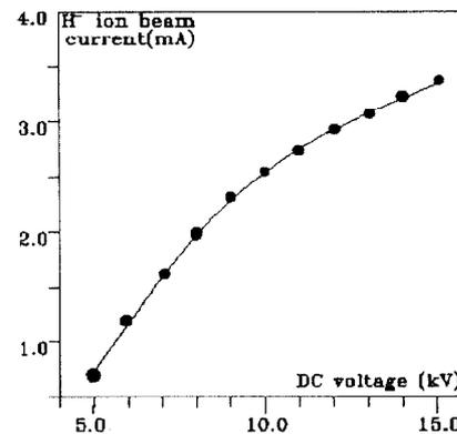
Figure 4.  $H^-$  ion beam current as function of extraction DC voltage for constant magnetic field  $B=0.65T$  at the discharge power of 210V, 3.5A, converter potential  $U_{conv.}=20V$  and gas flow  $Q=8cm^3/min$
