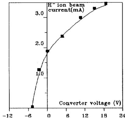
Figure 2.  $H^-$  beam current as function of converter potential for constant magnetic field  $B=0.65T$  at the discharge power of 210V, 3.5A, gas flow 8 cm<sup>3</sup>/min and extraction DC voltage  $U_{ext.}=13$  kV
