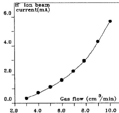
Figure 3. Relation between the extracted  $H^-$  ion beam current and the gas flow rate for constant magnetic field  $B = 0.65 T$  at the discharge power of 210V, 3.5A, converter potential  $U_{conv.}=20V$  and extraction DC voltage  $U_{ext.}=13$  kV
