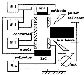
Figure 1. Experimental arrangement for the modified negative ion source.
