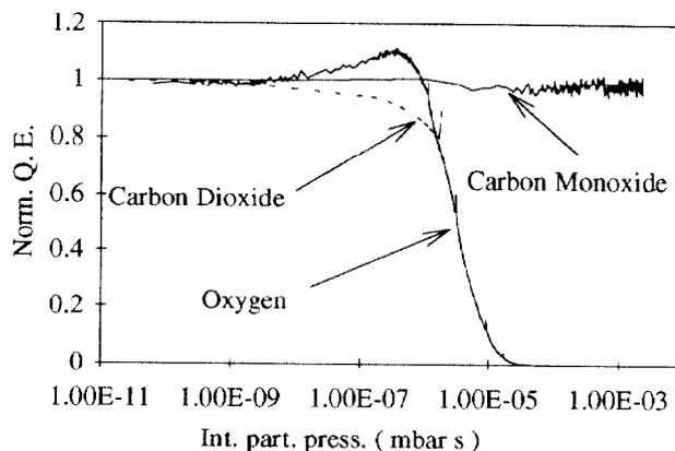
Fig. 6. Poisoning of KCsSb cathode with different gases.
