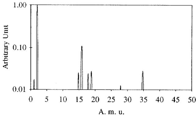
Fig. 2. Preparation chamber residual gas composition, for a total pressure of  $3 \cdot 10^{-11}$  mbar.
