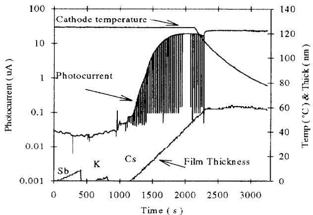
Fig. 3. Preparation procedure of a KCsSb cathode: see text for more details.
