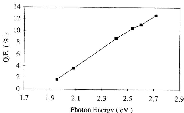
Fig. 5. Spectral response of a KCsSb photocathode.
