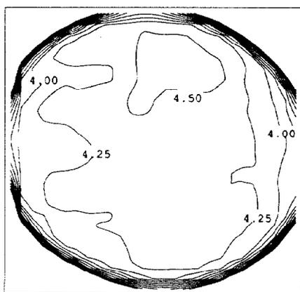
Fig. 4. QE spatial distribution over a KCsSb photocathode (30 mm diameter,  $\lambda = 543$  nm).
