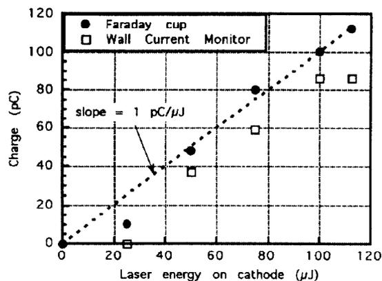
Figure 4: Charge vs. laser energy
