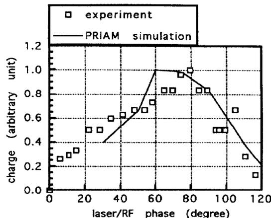
Figure 3: Charge vs. relative phase between laser and RF
