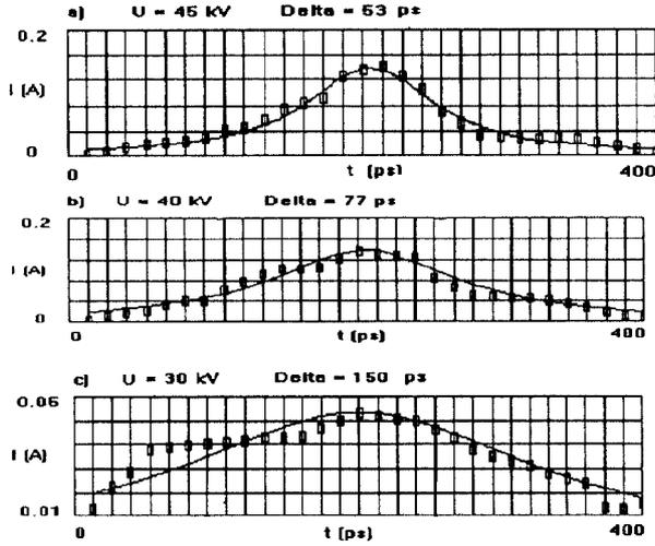
Figure 2: Shape of an electron bunch current at different energies: 45 keV (a), 40 keV (b), 30 keV (c) and at the same laser pulse parameters.
