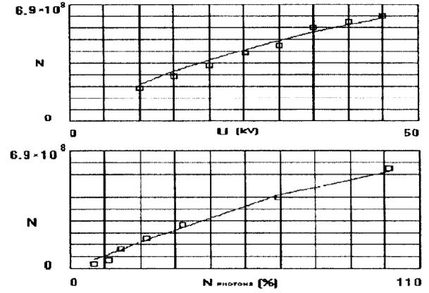
Figure 3: Total number of electrons in the bunch as a function of bunch energy (a) and number of photons in laser pulse (b).
