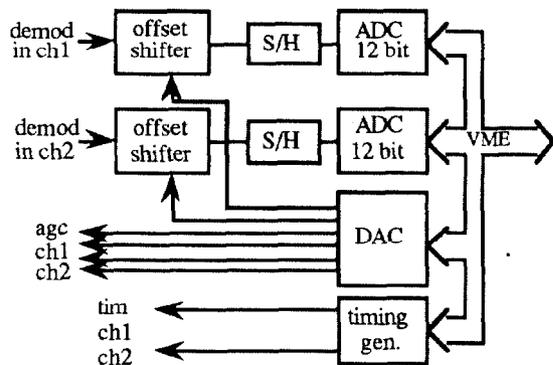
Fig. 3 Timing/ADC/DAC/bus
