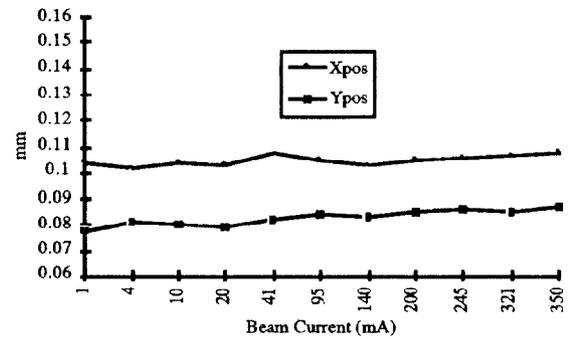
Fig 5 BPM position versus beam current
