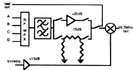
Fig. 1 BPM detector RF part
