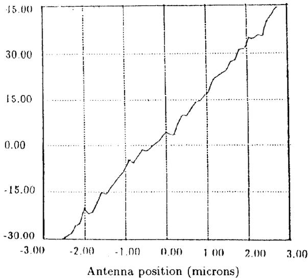
Figure 6. Transmission voltage through BPM versus antenna position (1 chanel= $2.5 \cdot 10^{-13}$  Coulomb).
