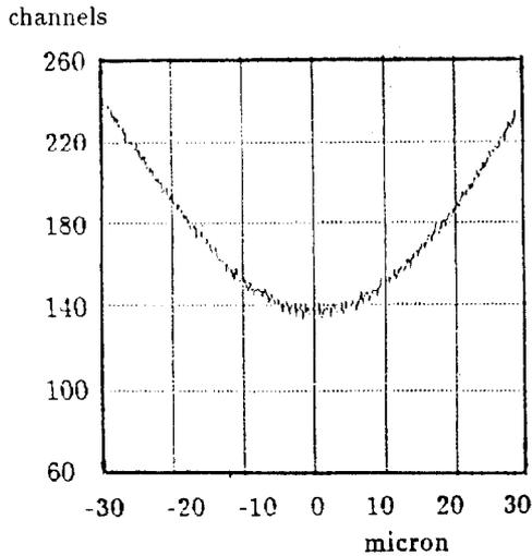
Figure 5. Amplitude BPM output for different antenna position (1 channel=  $2.5 \cdot 10^{-13} C$ )
