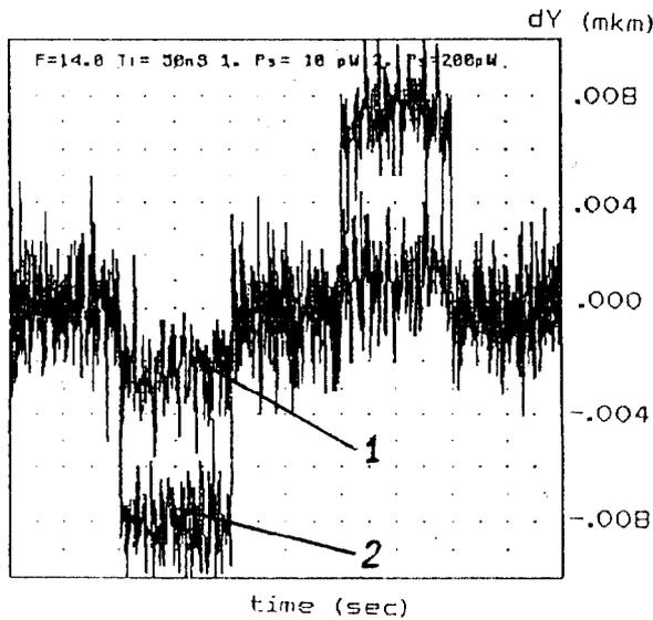
Figure 2. The results of measurement of electronics sensitivity. 1 - input power= $2 \cdot 10^{-10}W$ , 2 - input power= $10^{-11}W$
