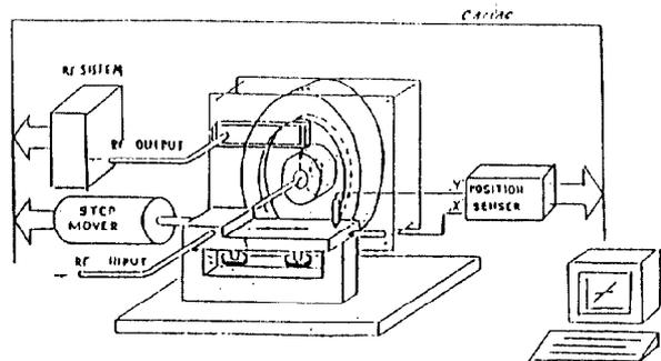
Figure 4. Test setup of BPM.
