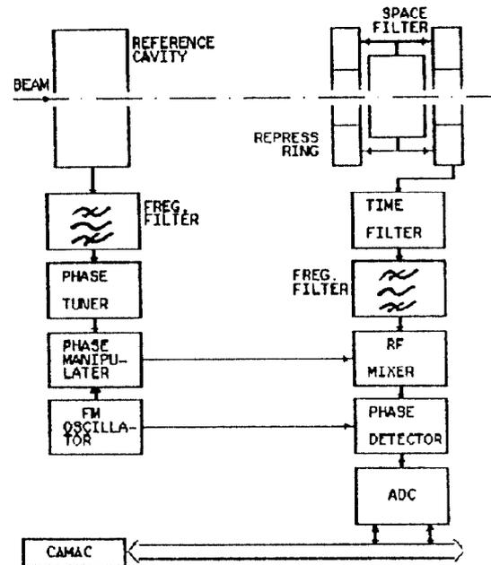
Figure 1. The block diagram of the electronics of BPM
