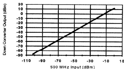
Figure 3. Response of Down Converter Stage (IF = 500kHz)
