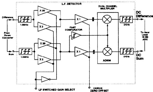
Figure 4. Dual Channel Low Frequency Detector
