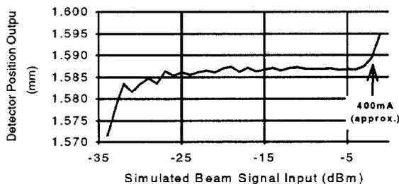
Figure 5. LabVIEW® Automated Data Processor Response
