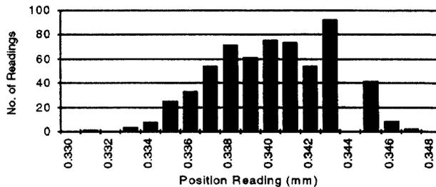
Figure 6. With-Beam Data Showing Typical Noise (BPM H9)
