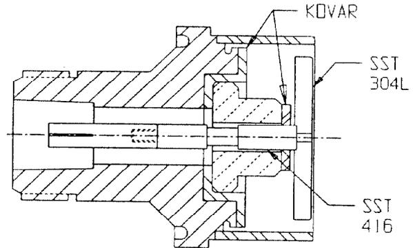
Figure 3: BPM Feedthrough
