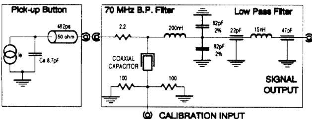
Fig. 2 : BP Filter schematics.
