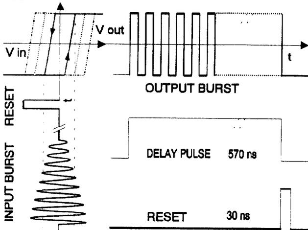
Figure 3 : Limiter Operating Principle.
