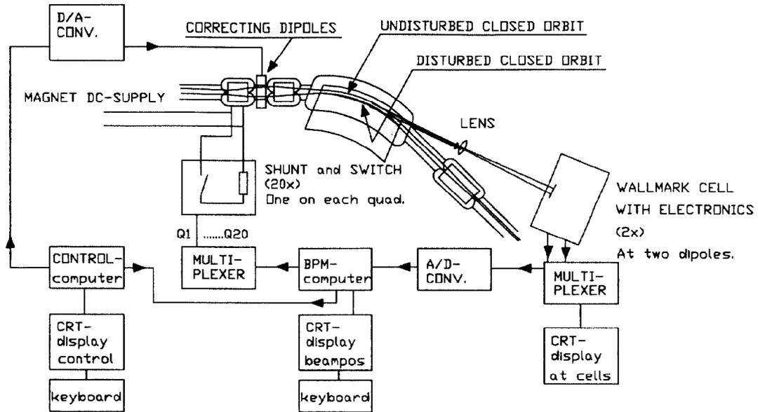
Fig. 1. Block schematic of the measuring system.
