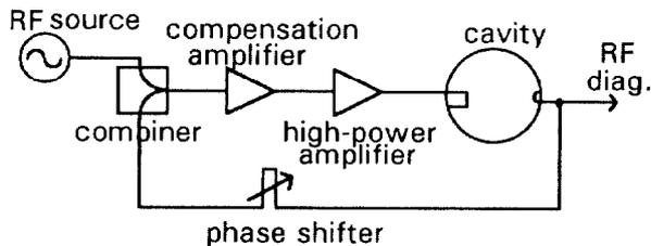
Fig. 1. Direct RF feedback on an accelerator.
