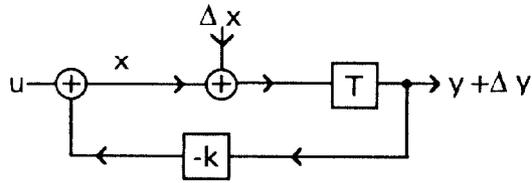
Fig. 2: Mathematical representation of the RF loop. The non-linear transfer function  $T$  has been adjusted in a way that  $T(x)=x$  for the working point  $x$ .
