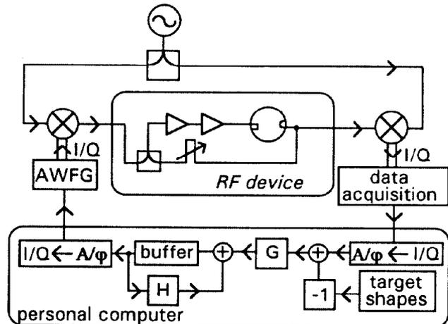
Fig. 3 Adaptive feedforward RF system.
