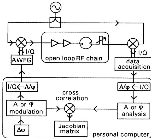
Fig. 4. Measurement of an RF device transfer function.
