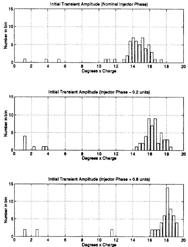
Figure 5. The system can be used to record injection transients as an accelerator diagnostic. Histograms of the longitudinal transient amplitudes for three adjustments of injector phase.
