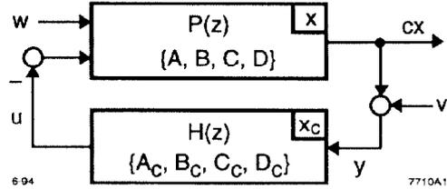
Figure 1. Block diagram of the LQG regulator problem.
