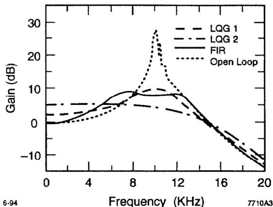
Figure 3. Frequency responses for four-bunch beam.
