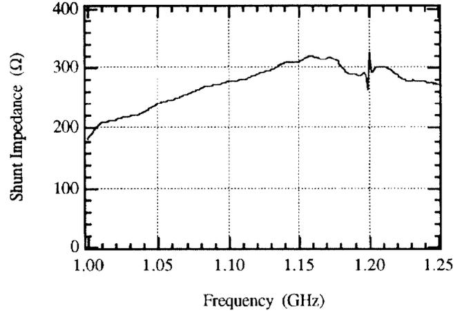
Figure 5. Longitudinal kicker shunt impedance
