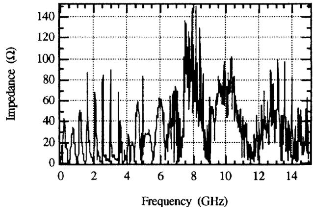
Figure 3. Transverse kicker beam impedance
