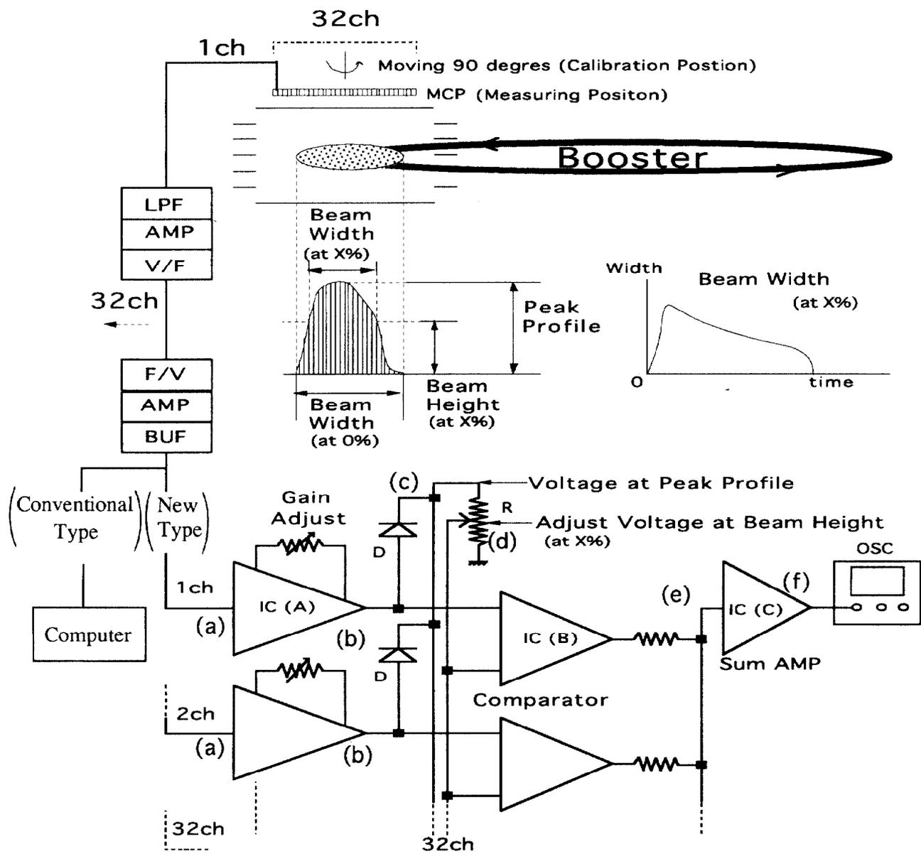
Figure 2. Conventional system for NDPM and new electric circuit for measuring the beam size in real time
