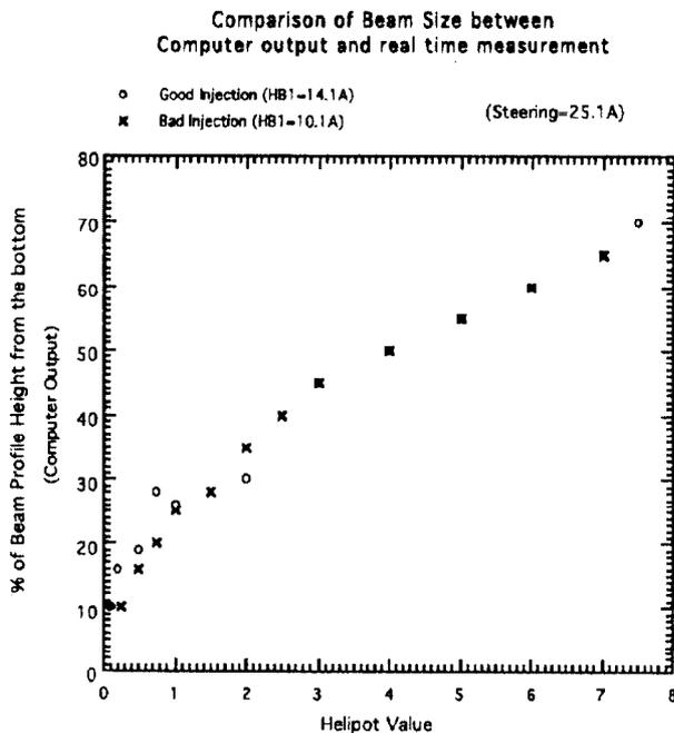
Figure 5. Relationship between the % of the peak height in the conventional system and the helipot value in the new system in order to obtain the same time dependence of the beam size.
