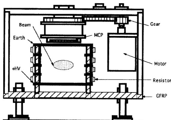
Figure 1. Plan of NDPM using an MCP
