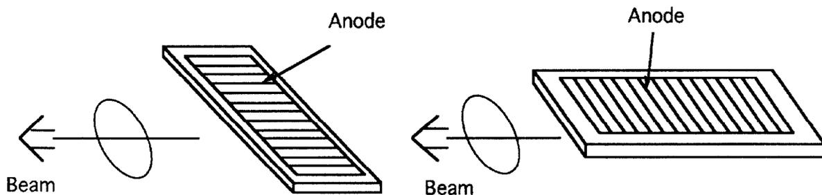
Figure 3. Relationship between the direction of the MCP anode and the beam (left, during the measurement; right, during the calibration)
