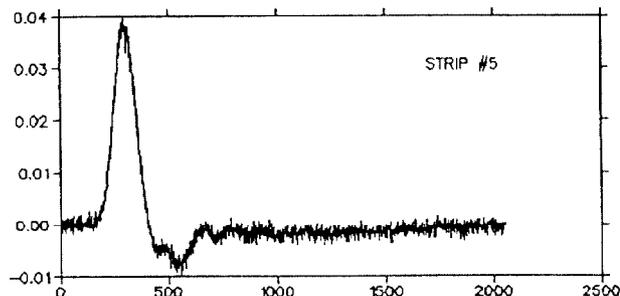
Fig.4: The wall current signal picked up by the multistrip monitor with RF background eliminated
