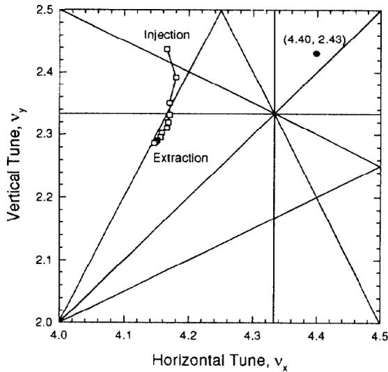
Fig. 3 Tune diagram indicating booster tune shift during acceleration
