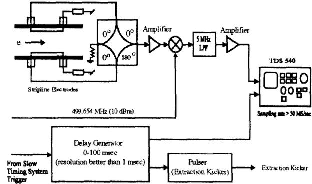
Fig. 1 Betatron tune measurement instrumentation system
