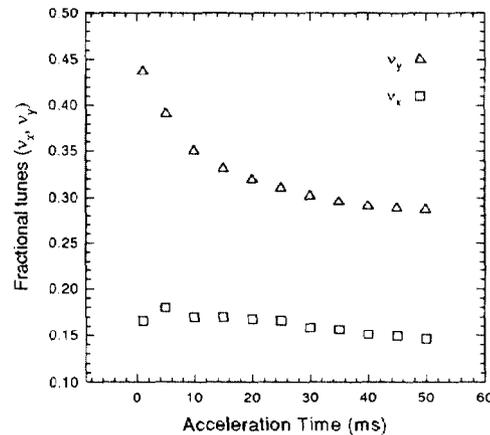
Fig. 2 Betatron tune of the accelerated beam
