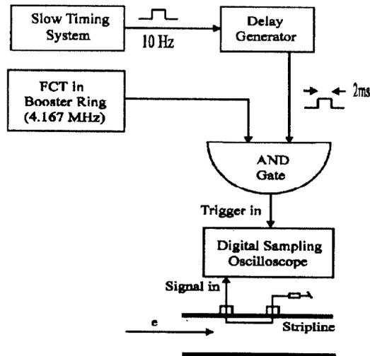
Fig. 4 Functional block diagram of the beam diagnostic system for bunch length measurement
