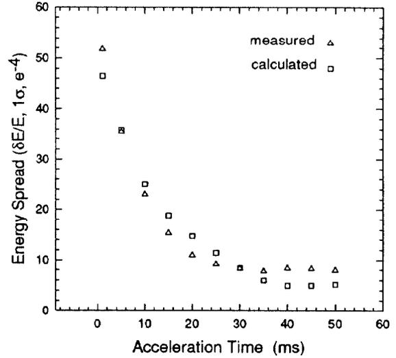
Fig.6 Energy spread during acceleration
