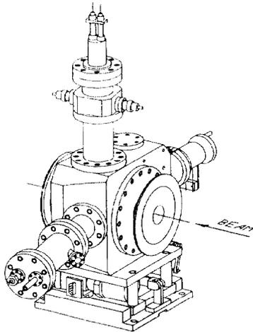
Figure 1. The CERN Bunch Length and Velocity Detector
