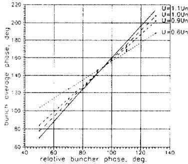
Figure 4. Bunch center vs buncher phase with buncher voltage as a parameter.
