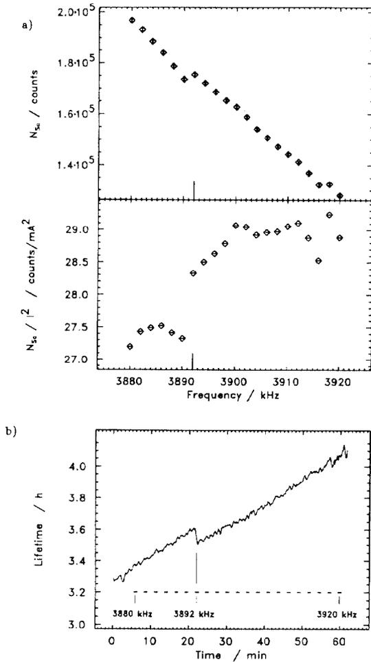
Figure 3: Example of an energy measurement. a) counts of scattered electrons: raw data upper, normalized data lower curve b) lifetime of the beam; the bars indicate the times when the depolarizer was active. In each case the step indicates depolarization after the depolarizer was set to 3892 kHz and frequency modulated by  $\pm 1.02$  kHz for 60 s.
