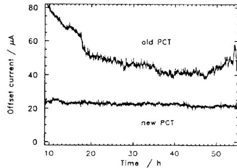
Figure 2: Drift and noise of the offset of the old and the new PCT at zero beam current within two days.
