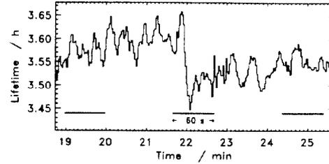
Figure 4: Lifetime during an energy measurement. The times when the depolarizer was active are indicated. When the depolarizer hits the resonance frequency full depolarization is reached after  $\tau_{Dp} \leq 20$  s.
