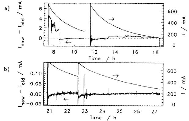
Figure 1: Comparison of the performance of the new and the old PCT a) without b) with RF-filters inserted in the interconnection wires of the sensor of the new PCT. The beam current  $I$  (right scale) and the difference between the signals of the old and the new PCT are displayed (left scale).
