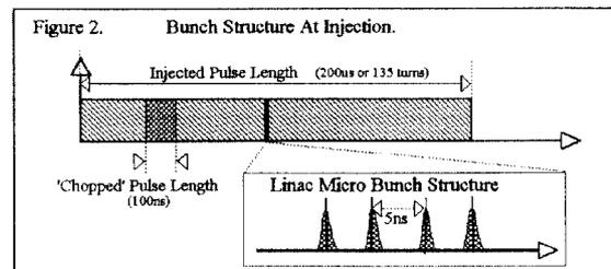
The 202.5 MHz linac provides a 200  $\mu$ s macro pulse length, composed of 1 ns micro-bunches, spaced by 5 ns. These debunch while drifting over 35.8 m, to a sinusoidally excited debuncher cavity, which is used to optimise momentum spread for the synchrotron. Particles then drift 16 m to the stripping foil where they enter the synchrotron.
