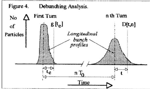
A particle starting at time  $t_e$  relative to the bunch centre on the first turn (Figure 4), will arrive at time  $t$  on the  $n^{\text{th}}$  turn if  $\Delta T$ , the change in revolution time per turn due to momentum error, is such that:
