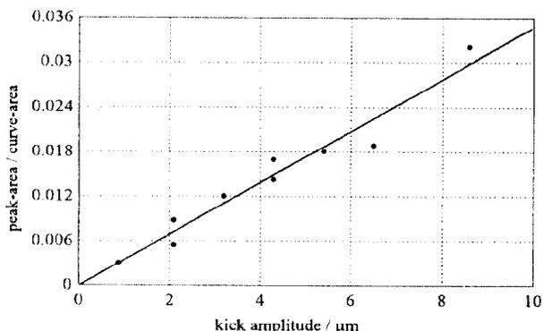
Figure 8. The relative beam loss depends linearly on the orbit kick amplitude (measured here at  $47.4 \text{ Hz}$ )
