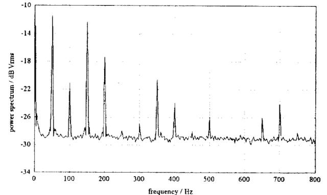
Figure 6. Frequency spectrum with a 350 Hz line
