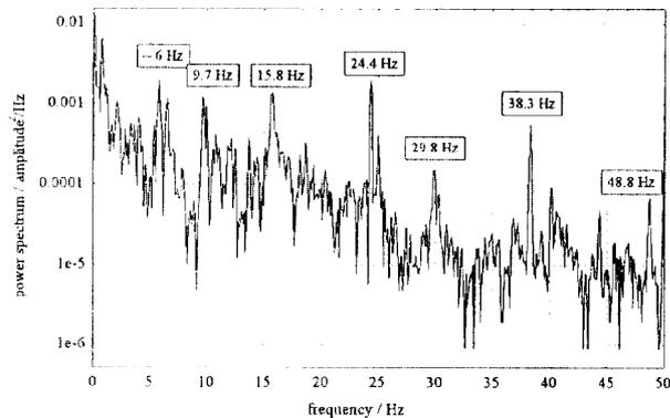
Figure 4. Spectrum of the ground or magnet motion
