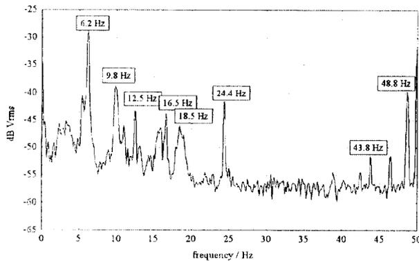
Figure 3. Frequency spectrum of the lost protons
