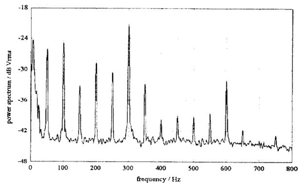
Figure 5. Frequency spectrum with a 300 Hz line
