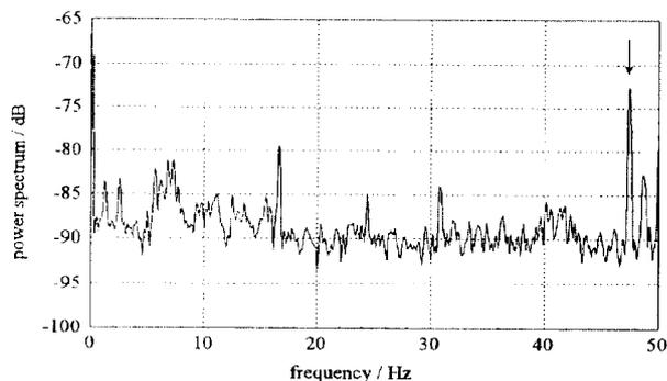
Figure 7. The beam loss spectrum during an artificial excitation of  $8.6 \mu\text{m}$  amplitude at  $47.5 \text{ Hz}$ .
