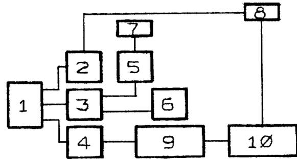
Fig.2. The block diagram of the system for monitoring the current and controlling the HF voltage across the dees: 1 - computer; 2 - ADC; 3 - counter; 4 - DAC; 5 - current integrator; 6 - synchronizer; 7 - beam current detector; 8 - amplitude detector; 9 - HF - generator, 10 - resonant system.
