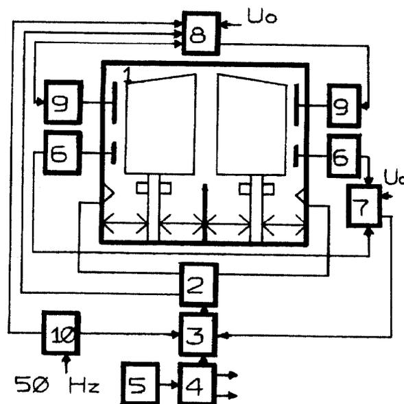
Fig.1. The block diagram of the KI cyclotron HF system: 1 - resonant system of cyclotron; 2 - HF oscillator PKV 250; 3 - HF controller; 4 - HF wide-band amplifier; 5 - master HF oscillator; 6 - capacitance-type HF dividers; 7 - error amplifiers with reference supply; 8 - regulator of the natural frequency of resonant circuits and the difference of the voltage at the dees; 9 - servoamplifiers; 10 - pulse oscillator.
