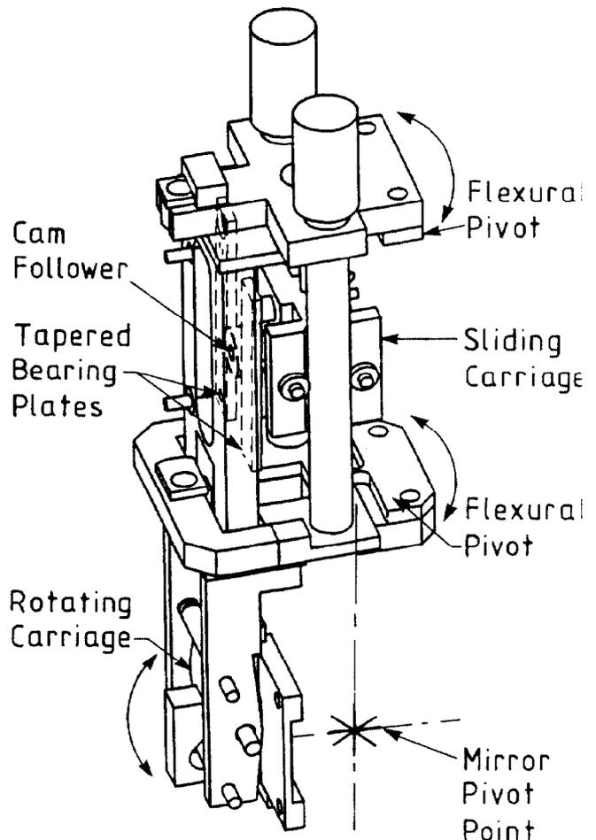
Figure 1. Rotation Mechanisms
