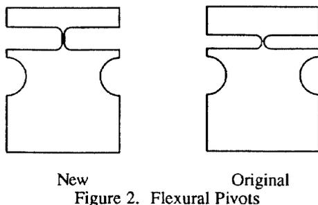
Figure 2. Flexural Pivots
