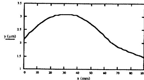
Figure 4. Profile Of Deformed Mirror Face
