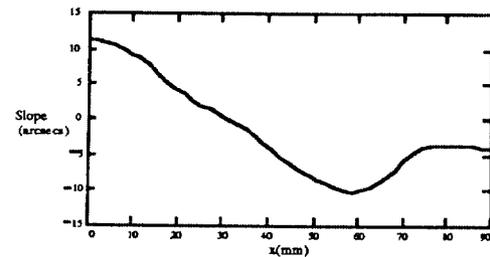
Figure 5. Slope Of Mirror Face
