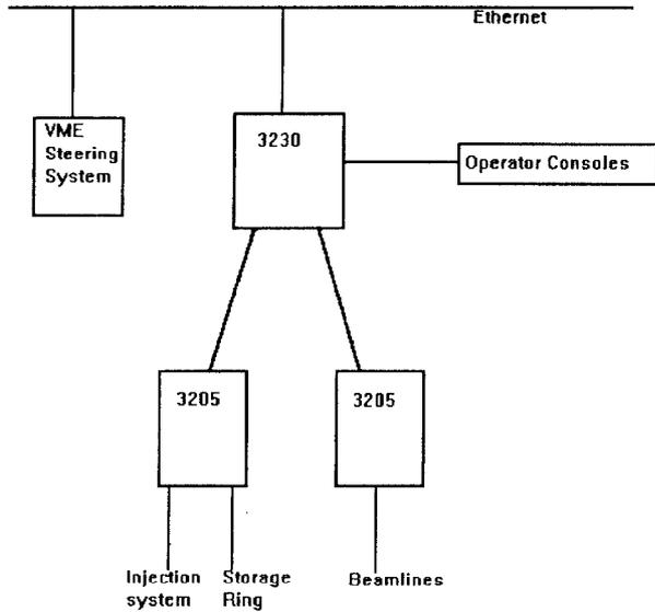
Figure 2. Control system after upgrade
