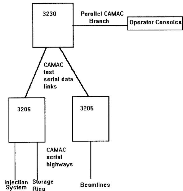
Figure 1. The SRS Control System
