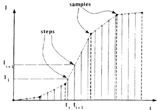
Figure 1. Example of samples and steps.
