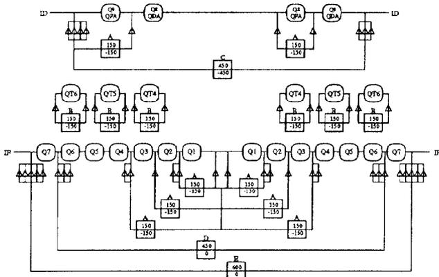
Fig. 1 Power supply configuration for IR quadrupoles.
