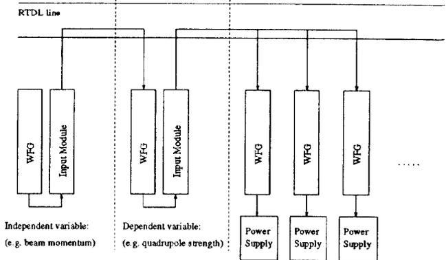
Fig. 2 Layout of the ramp control hardware.
