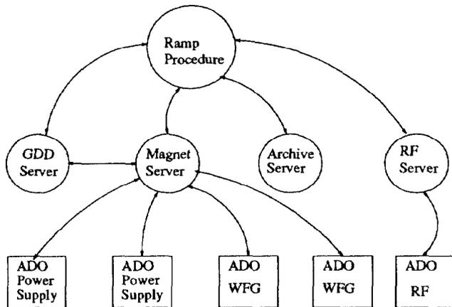
Fig. 3 Layout of the ramp control software.
