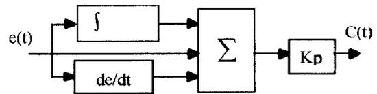
Figure 6. PID Algorithm & Block Schematic
