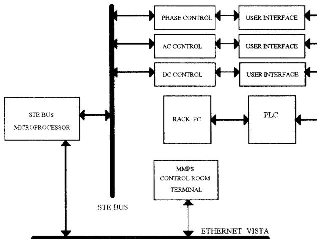
Figure 4. MMPS Digital Control System Schematic
