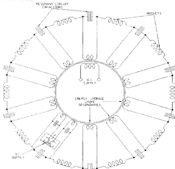
Figure 1. ISIS Ring Magnets 'White' Circuit Schematic
