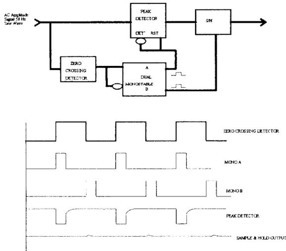
Fig 5. A.C. Amplitude Error Signal Generation.
