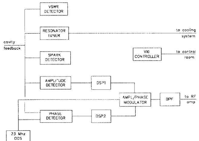
Figure 1. Cyclotron Control System Block Diagram
