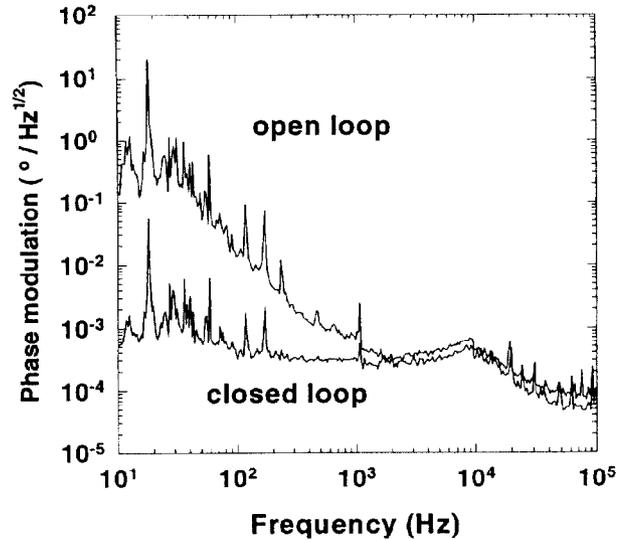
Figure 5. Residual Phase Noise
