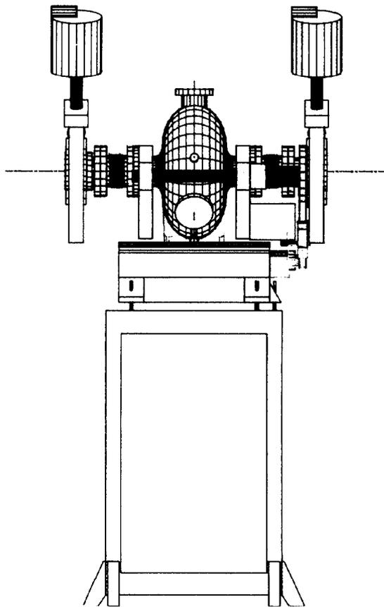
Fig1. RF cavity on the mechanical tuning cage, equipped with bellows and vacuum valves
