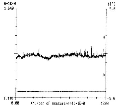
Fig.2 Measurement of phase (upper curve) of gap voltage on one cavity (no phase loop installed) with respect to the reference signal. The lower curve shows the ratio between the amplitudes of the two signals.
