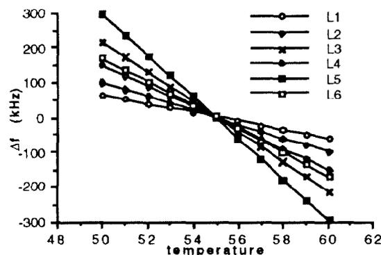
Fig. 1 Variation of the resonance frequency of the first six longitudinal modes vs. temperature (55°C taken as the reference). At 55 °C: L1=950.056 MHz, L2=1055.017 MHz, L3=1419.029 MHz, L4=1513.440 MHz, L5=1598.314 MHz, L6=1877.001 MHz
