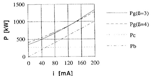
Fig. 1 Computed RF power required for  $V_c = 7.5$  MV.
