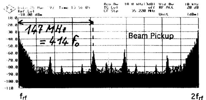
Fig. 3 Homogenous multibunch filling: 146.99 MHz side band of a longitudinal oscillation coupling to a 909.61 MHz longitudinal HOM of SR cavity number 3.
