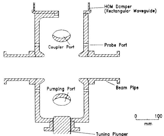
Figure 1: Cross-section of CESS-Upgrade RF cavity.
