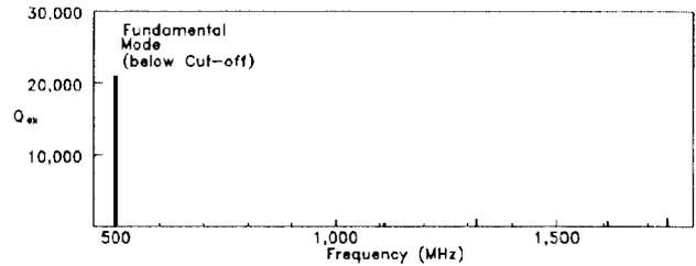
Figure 4: Mode spectrum of cavity with rectangular waveguide damper
