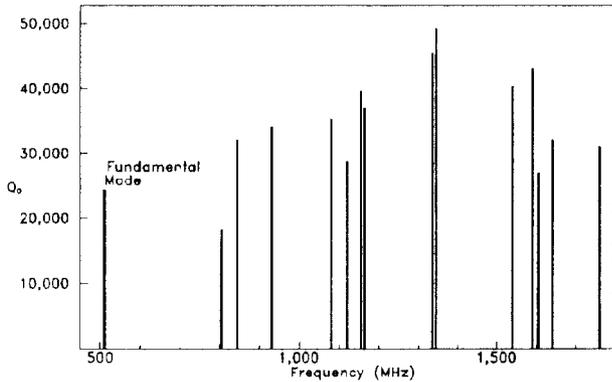
Figure 2: Mode spectrum of undamped cavity
