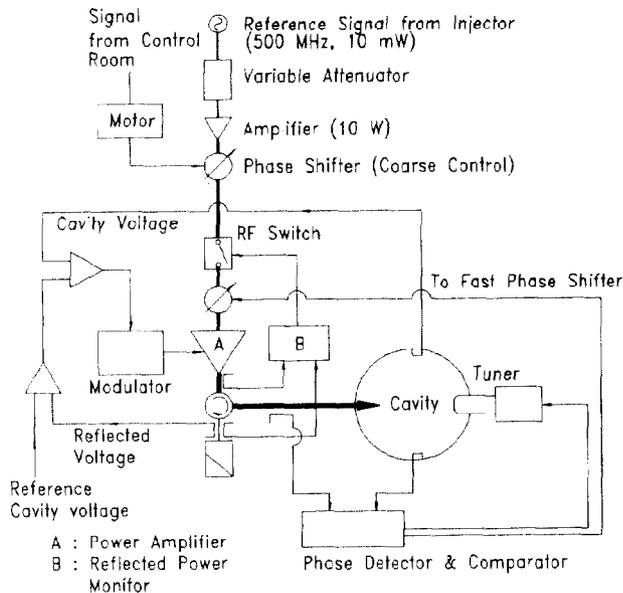
Figure 6: RF system of CESS-Upgrade
