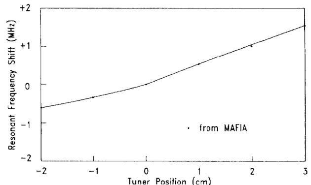
Figure 5: Resonant frequency shift as a function of tuner position
