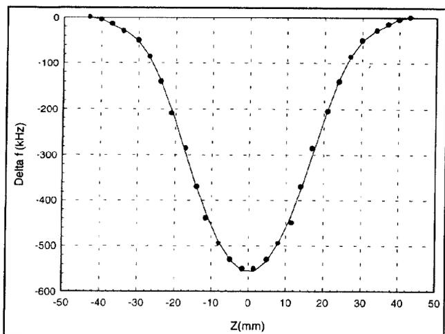
**Figure 1** Bead-pull of  $TM_{010}$  mode along axis of RF cavity with 1.0 mm diameter, 3.5 mm long metal bead giving a cavity R/Q of 50.2  $\Omega$
