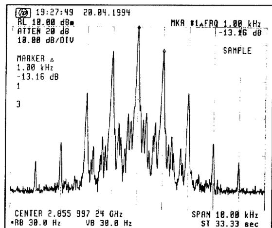
Figure 3 Narrow-band RF spectrum of cavity with 50% AM and I/Q RF feedback loop open.
