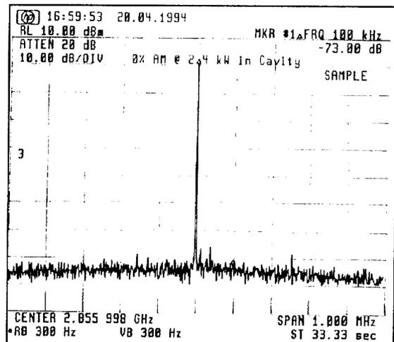
Figure 2 Wide-band RF spectrum of cavity with unmodulated reference and RF feedback loops closed
