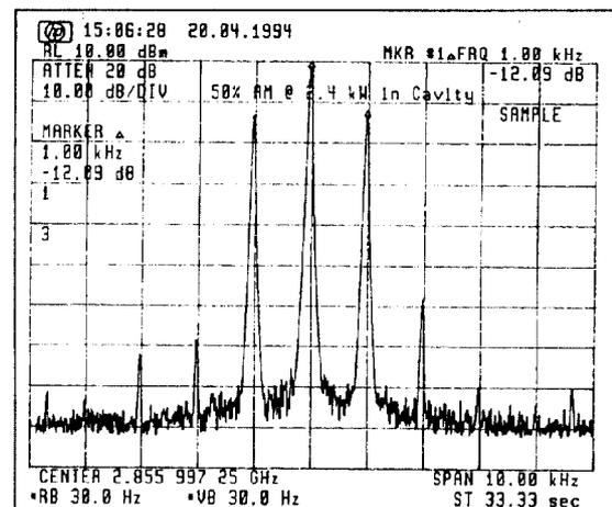
Figure 4 Narrow-band RF spectrum of cavity with 50% AM at 1 kHz and I/Q RF feedback loop closed.
