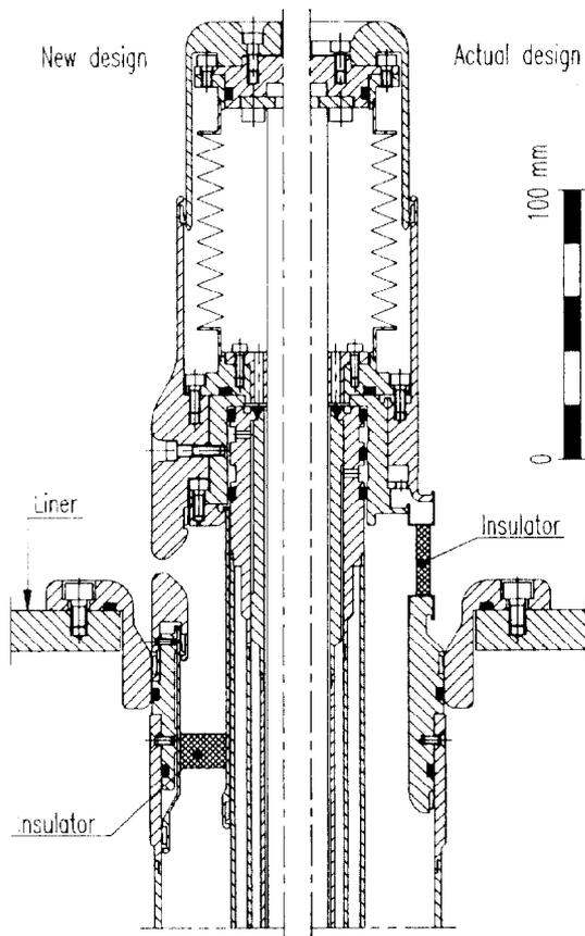
Fig. 1 Schematic drawings of the two couplers: the actual one (right) and the new modified version (left).
