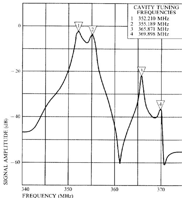
Figure 2. Swept Response to show Cavity Tuning Pattern
