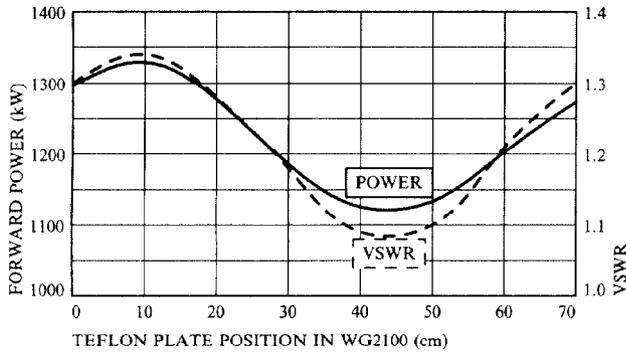
**Figure 3.** Variation of Output with Teflon Plate Position
