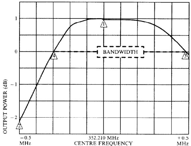
**Figure 5.** Bandwidth Response at 100 kV, 20 A
