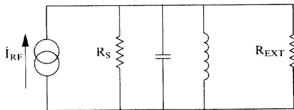
where  $R_S$  represents all the internal shunt resistance and  $R_{EXT}$  is the transformed value of the load resistance.
