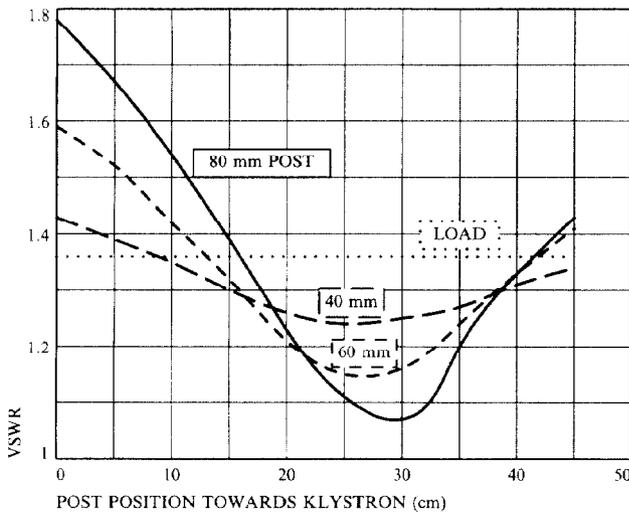
**Figure 4.** Variation of VSWR with Post Position (Measurements taken with a cold load)
