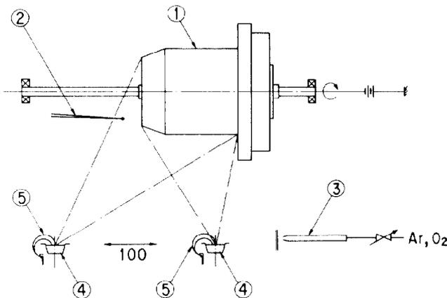
Figure 4. Setup of vacuum coating of  $\text{Cr}+\text{CrO}_x$ :
