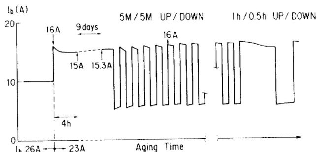
Figure 3. Heater aging in current up and down mode.
