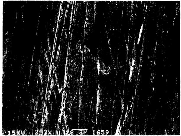
Figure 5. A SEM photo of  $\text{Cr}+\text{CrO}_x$  layer on Cu anode.
