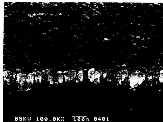
Figure 1. A SEM photo of columnar structure of TiN.
