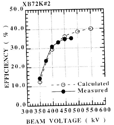
Fig-2)High power test results of XB72k#1
