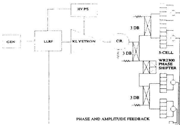
Figure 1: Synchrotron rf block diagram
