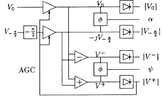
Figure 1: Probe signal processing board
