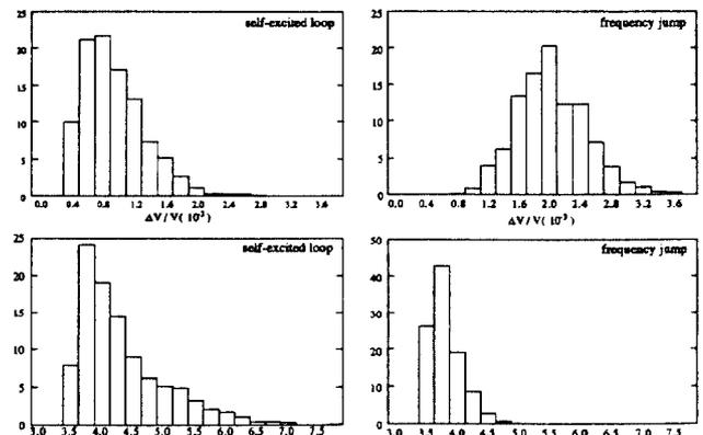
Figure 4: amplitude (top) and phase (bottom) histograms with K and  $\tau_m$  spreads for self-excited loop (left) and frequency jump (right) methods
