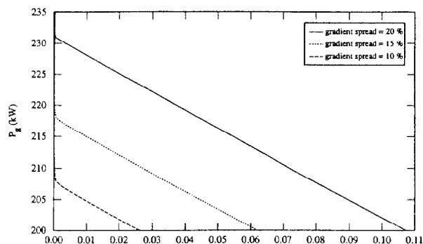
Figure 5: Needed source power (in kW) vs. the fluctuation level of the total voltage
