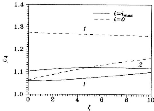
Figure 4: VSWR at the hybrid input port with beam loading  $\xi_1=16$ ,  $\beta_1=12.3$ ,  $\Delta\beta=0.5$ ,  $\rho_3=1.1$ ,  $\phi=5^\circ$ ,  $\phi_s=73^\circ$ . Curves 1:  $\Delta\xi = 0.5$ , curves 2:  $\Delta\xi = -1.7$
