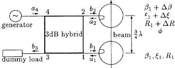
Figure 2: Network of two cavities driven by a 3 dB hybrid.
