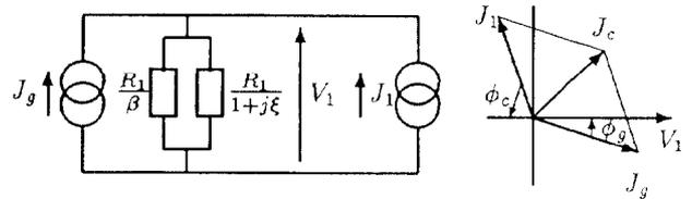
Figure 1: Equivalent circuit and phasor diagram.
