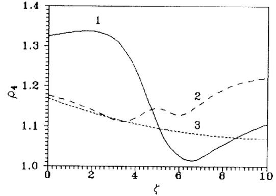
Figure 5: VSWR at the hybrid input port without beam loading  $\xi_1=0$ ,  $\beta_1=1$ ,  $\rho_3=1.1$ ,  $\phi=5^\circ$ ,  $\phi_s=73^\circ$ . Curve 1:  $\Delta\xi=0.2$ ,  $\Delta\beta=0.2$ , curve 2:  $\Delta\xi=-0.25$ ,  $\Delta\beta=0.2$ , curve 3:  $\beta_1=6.1$ ,  $\Delta\xi=0.2$ ,  $\Delta\beta=0.3$
