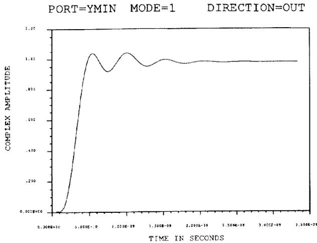
Figure 3: Envelope of  $S_{21}$  of the coupler in time domain.
