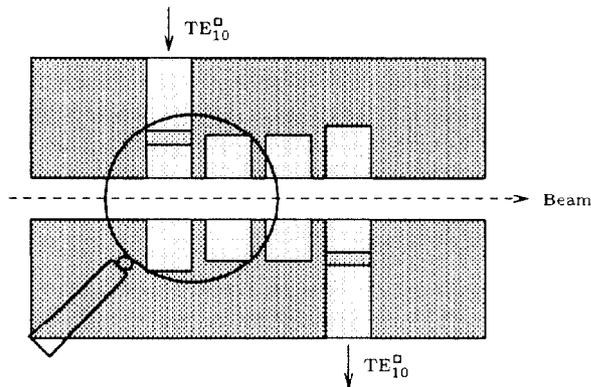
Figure 1: yz-cut of the mm-wave structure (scale 10:1). Both coupler cavities with waveguides, along with two cavities and the beam pipe are shown. The magnifying lens depicts the extension shown in more detail in Fig.2.
