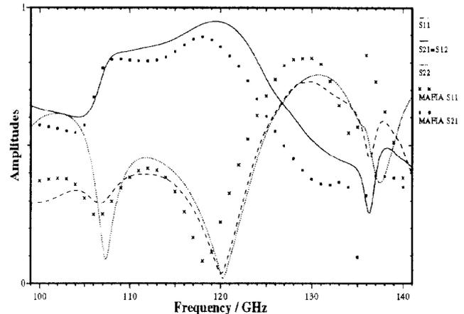
Figure 8: Transmission and reflection of the taper. Results from mode matching (220 modes) are drawn in lines, MAFIA (86 000 mesh points) as dots.
