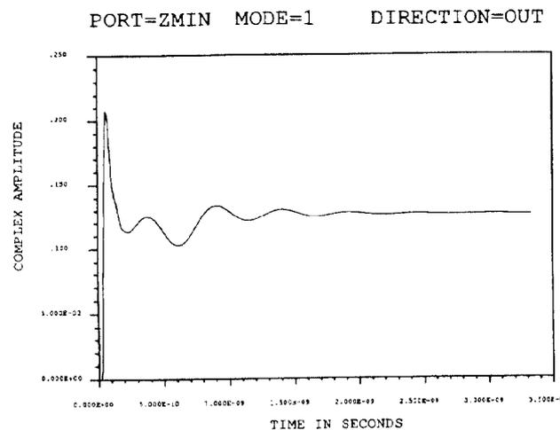
Figure 5: Envelope of the lowest port mode of the coupler at  $z_{min}$  in time domain (lost to the beam pipe).
