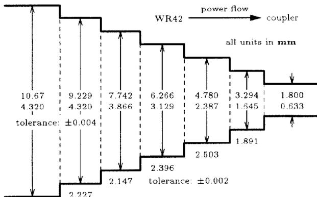
Figure 7: Dimensions of the taper. Tolerances are for  $\Delta S_{11} \leq 0.01$ . Required bandwidth: 2 GHz.
