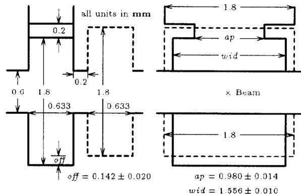
Figure 2: Dimensions of the unsymmetrical input coupler. Tolerances are for  $\Delta S_{21} \leq 0.01$  from MAFIA runs with 80 000, 100 000 and 120 000 mesh points.
