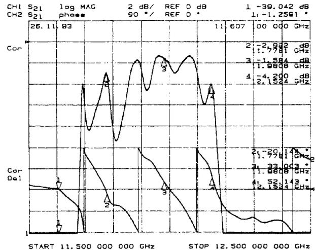
Figure 6: Measured amplitude (above) and phase (below) of  $S_{21}$  of a 10:1 scale model. The cursors are set (0,  $\pi/3$ ,  $2\pi/3$  and  $\pi$ -modes) from a previous  $S_{11}$  measurement.
