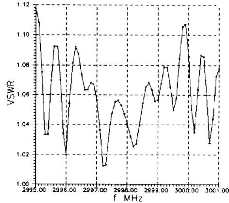
Figure 5: The impedance characteristic of 6m length accelerating section when the cells frequencies and coupling coefficients have homogeneous dispersion
