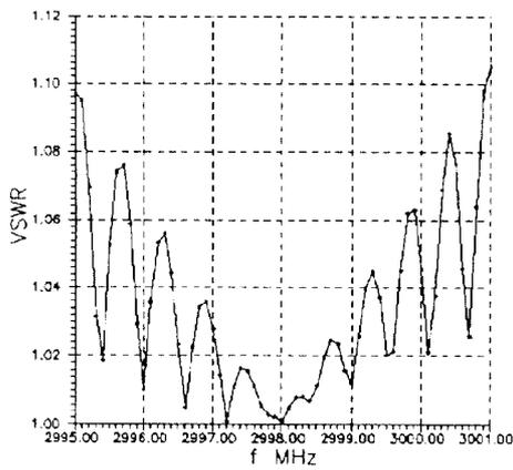
Figure 4: The impedance characteristic of 6m length accelerating section with ideal tuned cells and matched couplers
