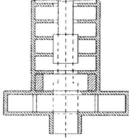
Figure 2: Schematic drawing of experimental model for measurement of the coupler parameters ( $f_c$ ,  $Q_{CL}$ )
