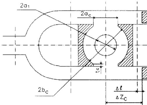
Figure 1: Symmetrical coupler with two waveguides and power divider
