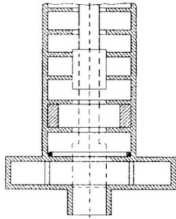
Figure 3: Schematic drawing of experimental model for measurement of the first DLW cell parameters ( $f_{r1}$ ,  $\frac{k_c}{2}$ )
