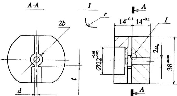
Figure 1. Construction of coupler.
