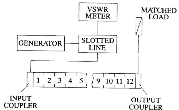
Figure 2. Experimental setup for matching coupler.
