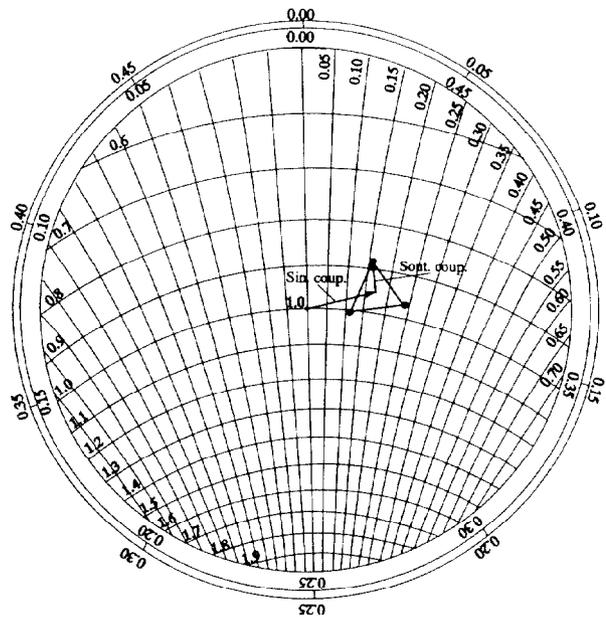
Figure 3. Smith chart ( $VSWR \leq 2$ ) with illustration of determining VSWR of input and output couplers.
